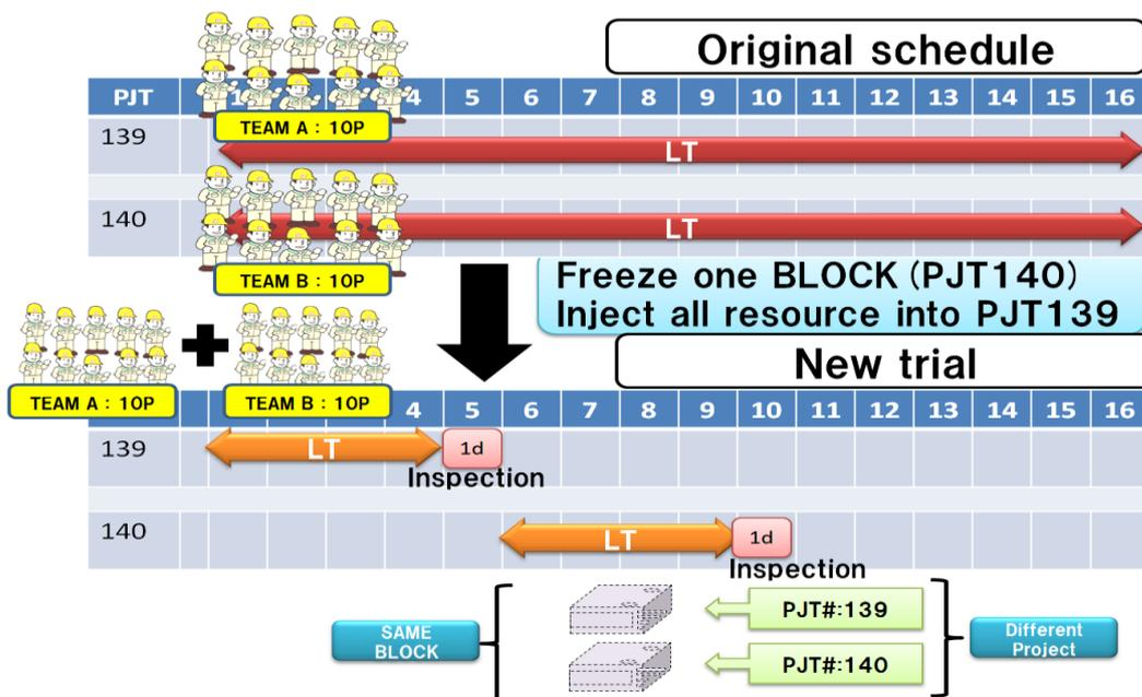
Fig. 4 Result of small experiment with TOC flow management in one of Indonesia’s shipbuilding company.
